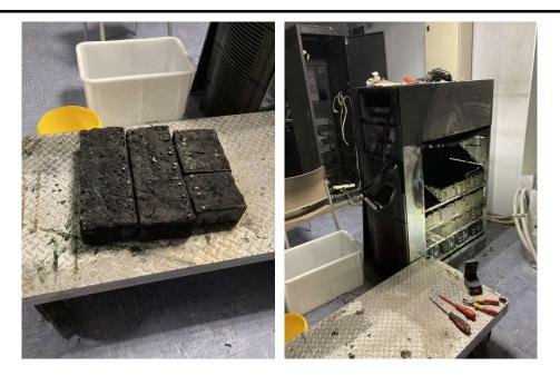
UPS fire incident at a UPS room in a Cinema Complex during the pandemic (November 2020) when the complex was shut down; the smoke detection early warning system went off hence the fire was extinguished by the security guards in time thus preventing the fire from spreading.
